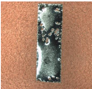
Figure 3: SnPb Soldering on Copper with centrotherm H 2 O Plasma
