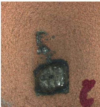
Figure 6: SAC Soldering on Copper without centrotherm H 2 O Plasma
