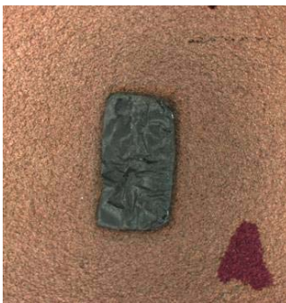
Figure 4: SnPb Soldering on Copper without centrotherm H 2 O Plasma
