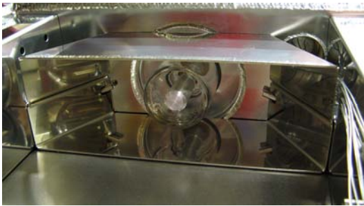
Fig. 4: Cooled and Encapsulated MW Plasma Head
