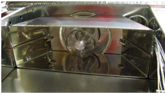
Fig. 4: Cooled and Encapsulated MW Plasma Head
